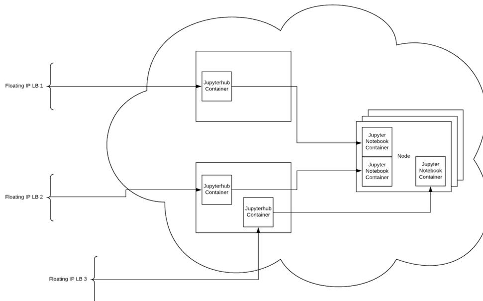
Additional Jupyterhub instances with differing configurations can co-exist on one cluster, noting that they are logically segregated.
