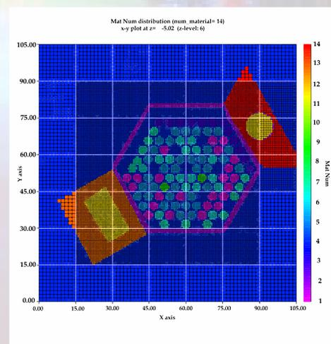
Fig. 1. Cross section of a 3-D deterministic radiation transport model used for a PENTRAN calculation on NOTCHPEAK for determining reactor critical flux.
