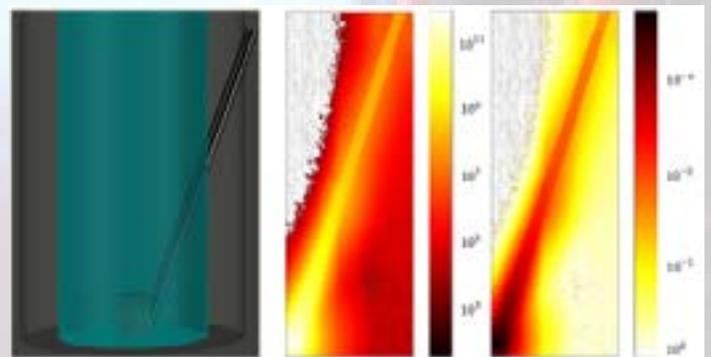
Fig. 3. (a, left) angular neutron profile of neutrons emerging from new beamline design for the UUTR. (b, right) CAD model and overlay of Monte Carlo results depicting neutron beamline; CHPC results.
